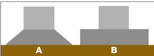
Fig.5 - Both construction methods for two-stepped walls are possible if the view from above is interpreted correctly. Both are common in the Mediterranean region. [Graphic: H.-J. Ulbrich]
